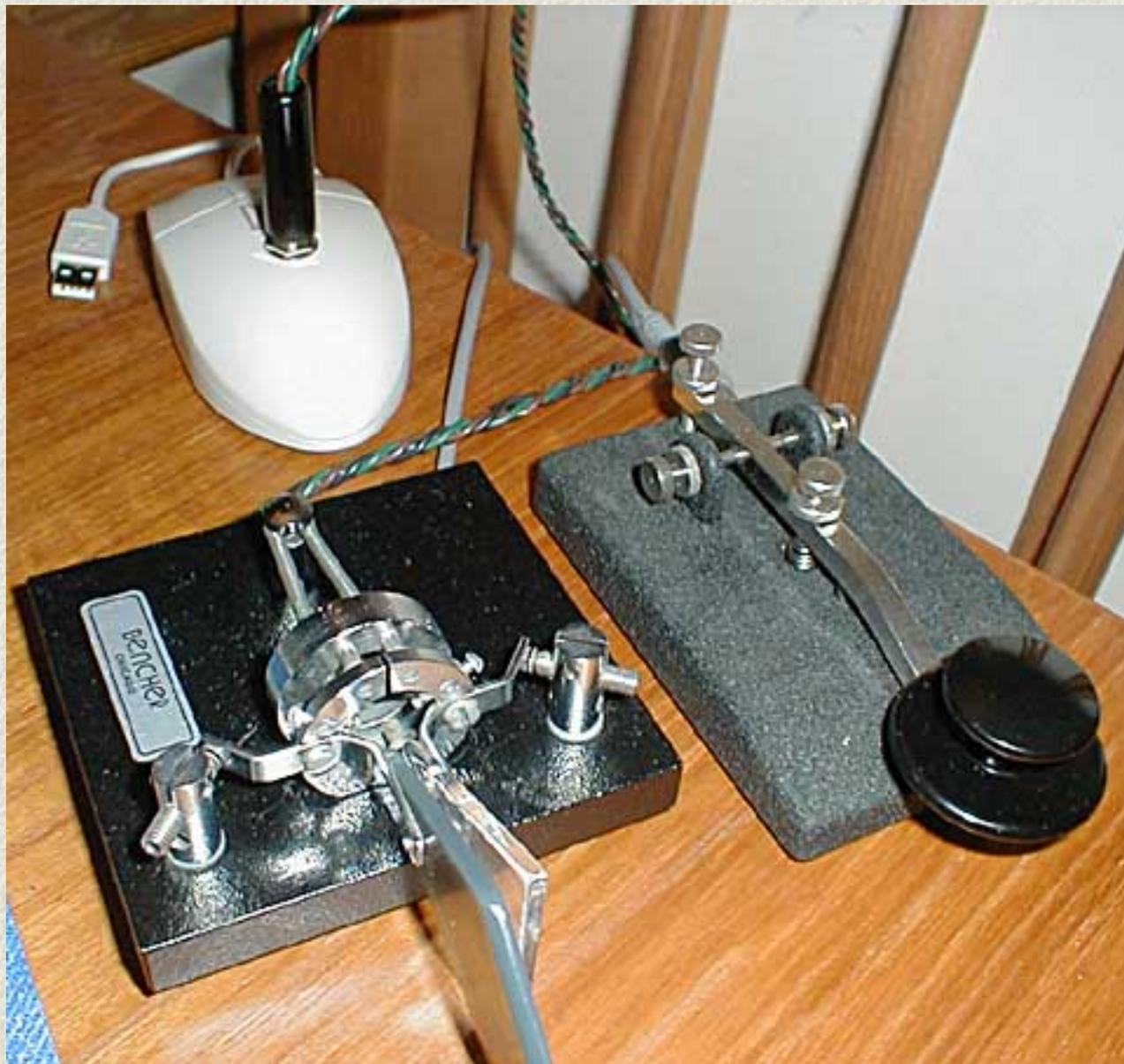
(You might notice that I have modified the Bencher paddles to mount inside the levers to give the narrower spacing I happen to prefer. Also, the dot paddle is custom built to stick out further to accommodate the fact that my thumb doesn't extend as far as my forefinger.)
